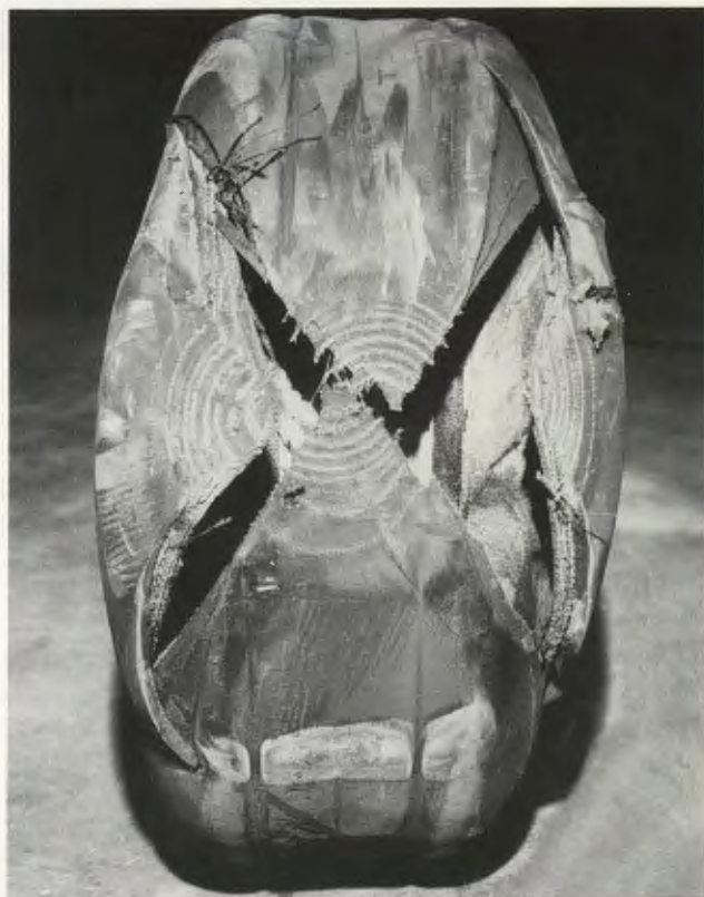
THE TIRE IMMEDIATELY FOLLOWING BLOWOUT.
