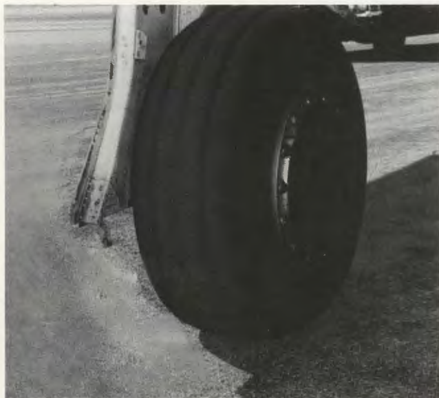
NOTE THE WORN SPOT WITH ALL CORDS EXPOSED.
